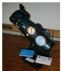
The telescope used in the Library Telescope Program is the Orion StarBlast 4.5-inch Astro Reflector Telescope, modified to provide durability for the telescope loaner program, is equipped with an 8- 24mm zoom eyepiece, and comes with supportive material.
